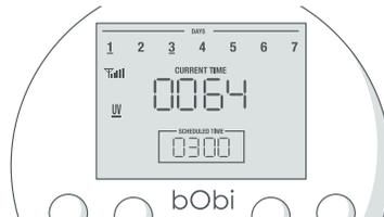
**Left Wheel:** While in mode 0300, the 4-digit number in the center of screen indicates the current of bObi's left wheel. Normal current ranges between 0020 and 0110.
