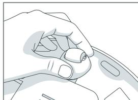
Dirt and dust on bObi's wall and edge sensors can reduce her performance. Regularly cleaning these sensors ensures that bObi keeps working at her best.
