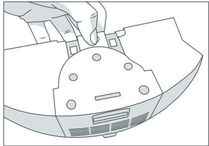
With the motor and filter removed, the dustbin may be washed with water.
