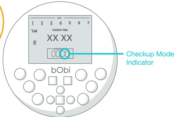
Press RGHT on bObi's remote to cycle through each step of the checkup test. Press LEFT to alternate between subsections of each step. The checkup mode indicator shows which step of the test bObi is in.
